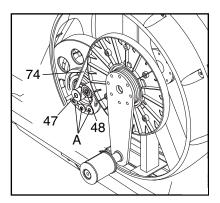
of the elliptical exerciser until the Belt (74) is tight. Then, tighten the three screws.
